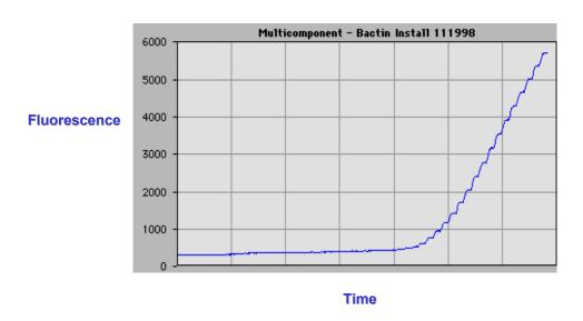
The combination of FRET and the 5'nuclease activity of AmpliTaq Gold® DNA Polymerase enables the 5' nuclease assay and the SDS instrumentation to collect data in real time. When the fluorescent signal Reporter increases to a detectable level it can be captured and displayed as an **Amplification Plot**, Figure 17.
